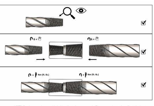
NOTE :Couplers must be assembled with calibrated torque wrench. Torque wrench must be calibrated at least every 24 months (+/- 15%).
